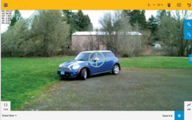
Camera view from SX10 within Capture for pointing cross hairs.
